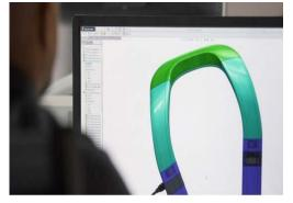
Car manufacturer Toyota has come up with a wearable device to aid visually impaired people in navigation. Called Project BLAID, the device is equipped with cameras to recognize objects around the user, and it will be worn around the user's shoulder. Vibration motors and speakers allow the device to communicate with the user, helping him in navigating his surroundings.
